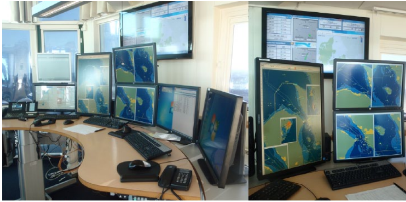
Figure 7. VTS workstation with VHF radio (far left), electronic chart with combined AIS/radar vessel targets (center/right), and meteorological data (top right). AIS = automatic identification system; VTS = vessel traffic services.
