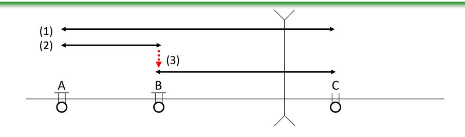
(1) Logic covering the overall warning zone(2) Train detection between A and B, B and C(3) Train tracking
