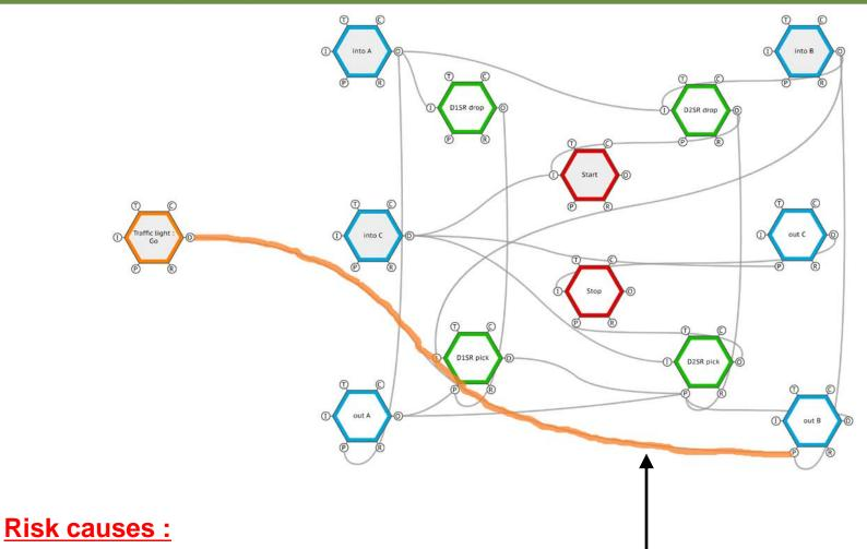
1. Control logic of railway crossing will collapse if this interaction(constraint) is broken.
